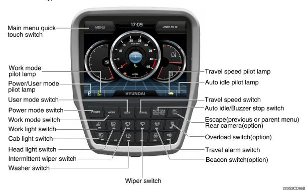
When some of the switches are selected, the pilot lamps are displayed on the LCD. Refer to the page 5-56 for details.
