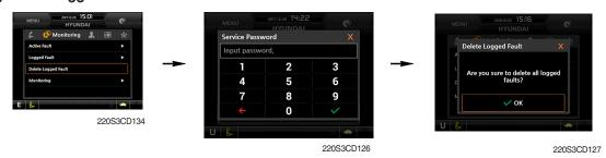
· The logged faults of the MCU, can be deleted by this menu.
