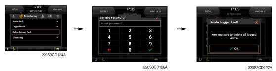
· The logged faults of the MCU and AAVM (option) can be deleted by this menu.
